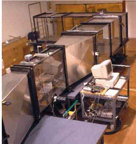
Figure 5. Wind tunnel to study droplet kinetics and thermodynamics in inlet ducts. This wind tunnel provides dynamic similarity to gas turbine inlets. Facilities such as these allow Mee Industries Gas Turbine Division to study and measure the practical aspects of droplet behavior in a real life setting
