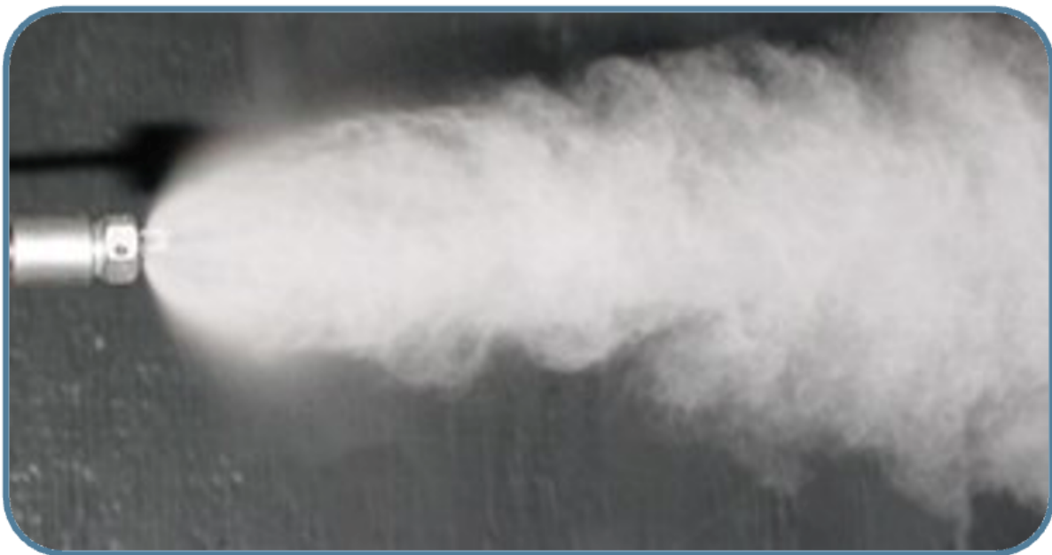
IP nozzle operating at 2000 psi (69 bar)
