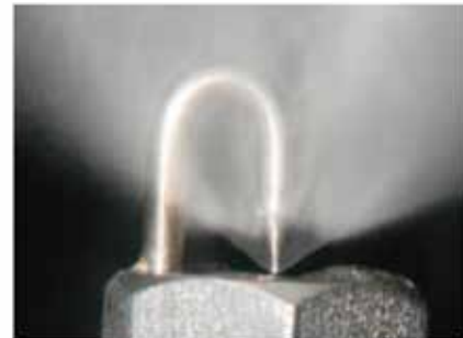
Figure 2. Conical Sheet formation and droplet break up with a MeeFog impact-pin nozzle operating at 2000 psi (138 bar). The flow rate is 0.045 gpm (0.17 L/min).
