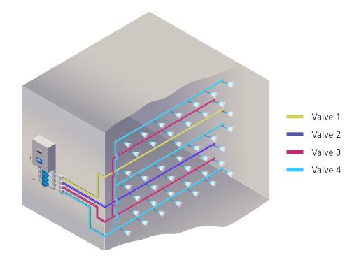
The MeeFog™ System can provide the precise control that your application requires. Valve Panels can be strategically located near the AHU. A single Pump Unit can supply high-pressure water to many Valve Panels thus providing precise humidity control to multiple AHUs.
