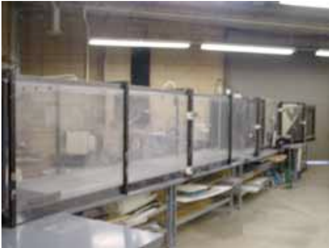
Figure 2. Experimental wind tunnel, 10.5m (34.5 ft.) long and capable of velocities up to 25 m/sec (4900 ft/min). Used to study droplet kinetics and thermodynamics under conditions similar to gas turbine inlet air ducts.
