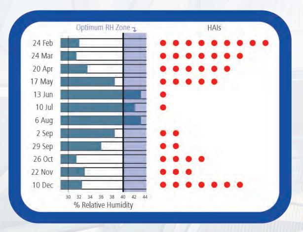
A study conducted in a new 250-bed academic hospital in the U.S. demonstrated the impact of RH on health. For more than a year, room temperature, absolute and relative humidity, lighting levels, room air changes, outdoor ventilation fractions, carbon dioxide levels, and room traffic were monitored in 10 patient rooms each hour. Of all metrics tracked, indoor RH most closely matched measured rates for HAI. As indoor RH was increased into the optimum range, patient HAI rates decreased.
