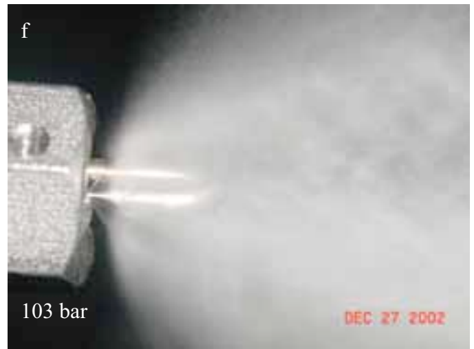
Figure 12. Sprinkle effect from a standard Mee nozzle at operating pressures from 34 bar to 103 bar (500 to 1500 psi). The views on the left are facing the impaction pin and on the right in line with the impaction pin. Note how sprinkle lessens with increasing operating pressure.
