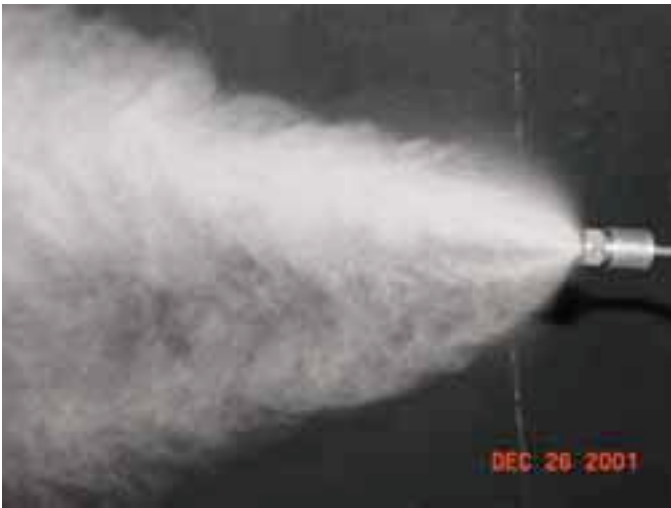
Figure 8. Distorted spray plume caused by intentional bending of the impaction pin, 138 bar (2000-psi) operating pressure.
