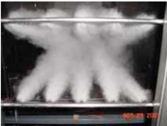
Figure 4. Fog nozzles manifold used to create saturated air in the wind tunnel. The use of a fog droplet filter makes it possible to achieve an airflow with very close to 100% RH.
