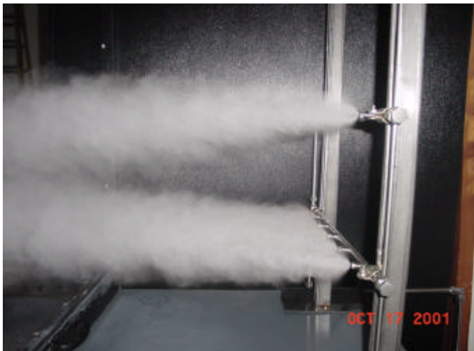
Figure 12. Side view of nozzle array; airflow velocity is 4 m/s (800 ft/min), operating pressure is 138 barg (2000 psig)
