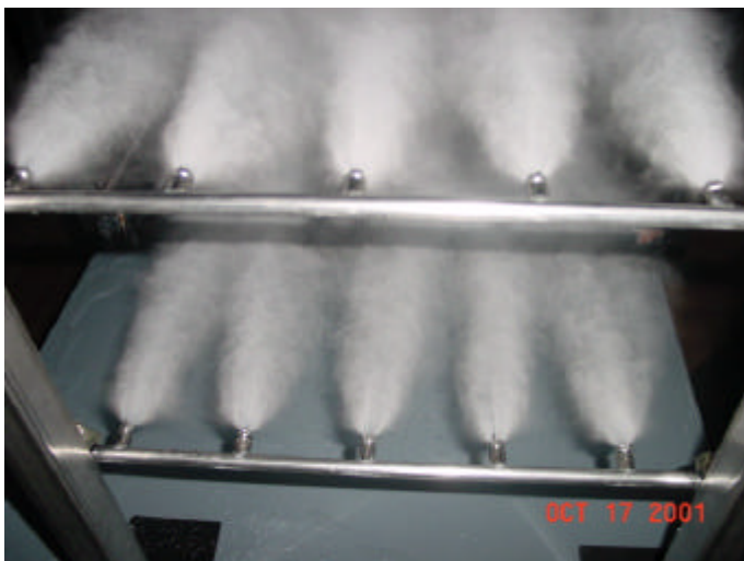
Figure 13. Face view of Nozzle Array; airflow velocity is 4 m/s (800 ft/min), operating pressure is 138 barg (2000 psig)
