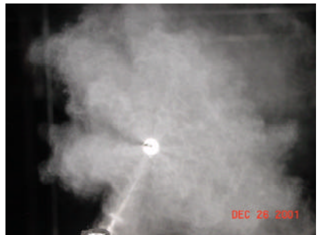
Figure 11. Counter-flow orientation of a fog nozzle in the wind tunnel; airflow velocity is 4 m/s (800 ft/min), operating Pressure is 138 barg (2000 psig)
