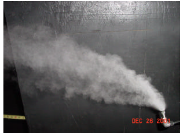
Figure 10. Ninety-degree orientation of a fog nozzle in the wind tunnel; airflow velocity is 4 m/s (800 ft/min), operating Pressure is 138 barg (2000 psig)
