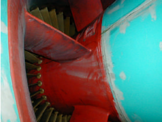
Figure 17. Intake cone and struts at an axial compressor inlet
