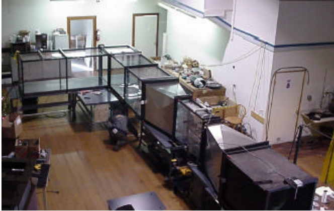
Figure 1. Experimental wind tunnel used for studying fog behavior in gas turbine inlet air ducts: 11 meter (36 foot) long, capable of up to 25 m/s (5000 fpm) airflow velocity
