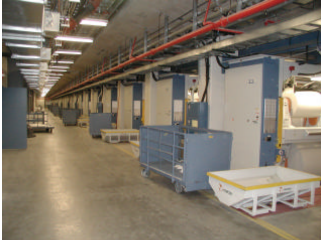
Reel Room Where Paper Rolls Are Automatically Fed Into The Bottom Of The Press
