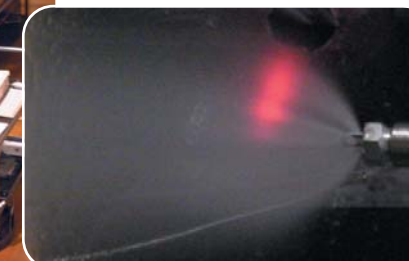
Mee Fog nozzle droplet sizing with laser particle analyzer instrument.
