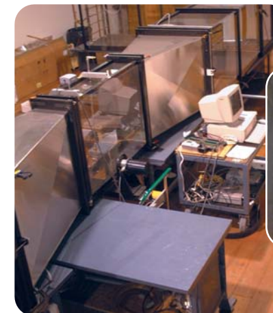
Wind tunnel used to study droplet kinetics and thermodynamics. Research & development facilities such as these set Mee Industries apart from the competition.
