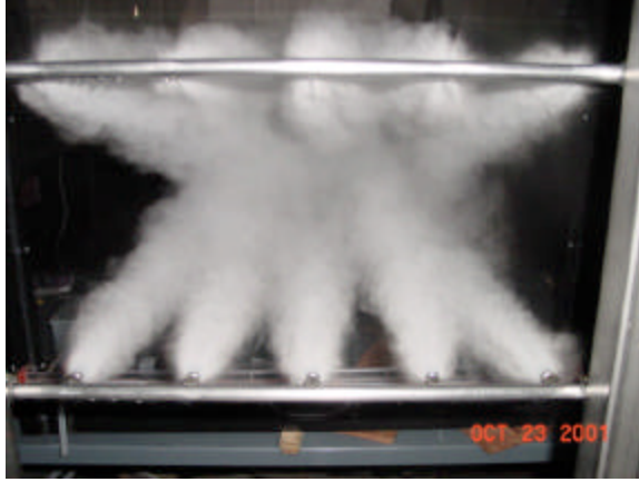
Figure 4, Fog nozzles manifold
